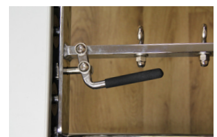
Fig 26b. Above Left is safe, above right is not engaged properly
